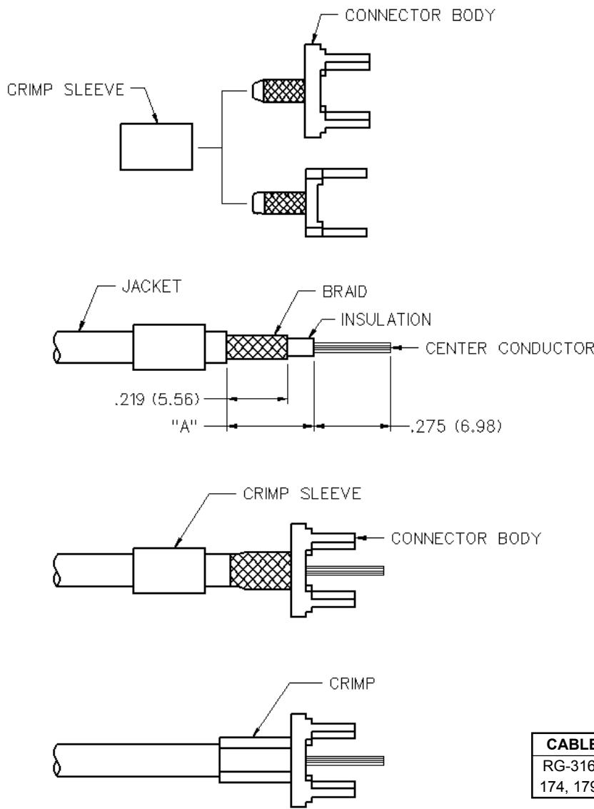
1. Identify connector parts. (2 piece parts)
