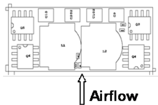
Figure 55. Airflow direction for thermal testing.
