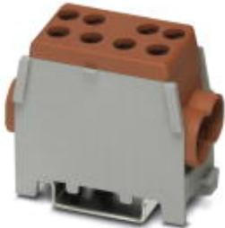
Trunk line branch terminal, nom. voltage: 400 V, nominal current: 125 A, connection method: Screw connection, Screw connection, number of connections: 4, number of positions: 1, cross section: 10 mm<sup>2</sup> - 35 mm<sup>2</sup>, AWG: 8 - 2, width: 27 mm, color: brown, mounting type: NS 35/7,5, NS 35/15
