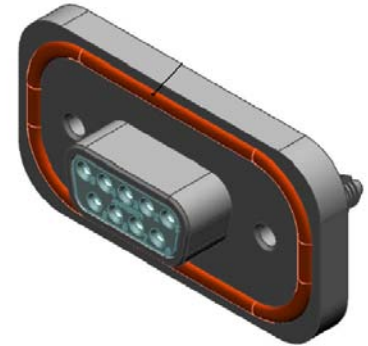
P/N MDB-E09SE-860 SHOWN 9 POSITION SOCKET, VERTICAL PCB TAILS WITH BOARDLOCK
