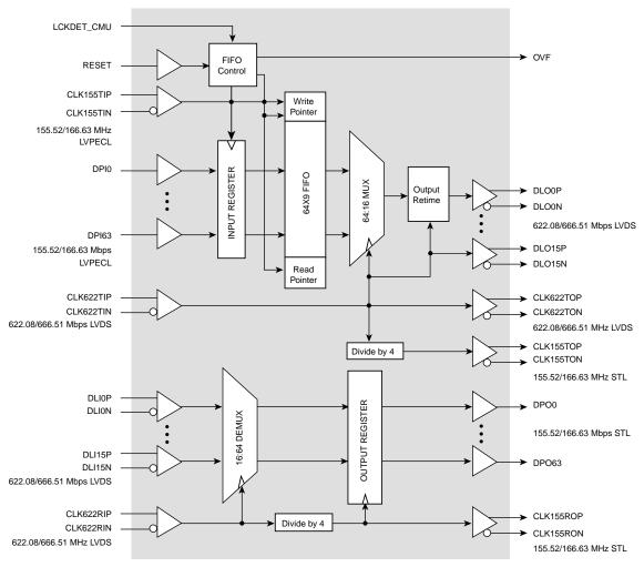
The **BCM8112** 16/64 LVDS/LVPECL interface is a fully integrated, 64:16 MUX and 16:64 DEMUX. The low-speed, 64-bit interface operates at 155.52/166.65 Mbps, and the high-speed, 16-bit interface operates at 622.08/644.45 Mbps. The 64-bit input interface is LVPECL, while the 64-bit output interface is STL. Both the 16-bit input and output interfaces are LVDS.
