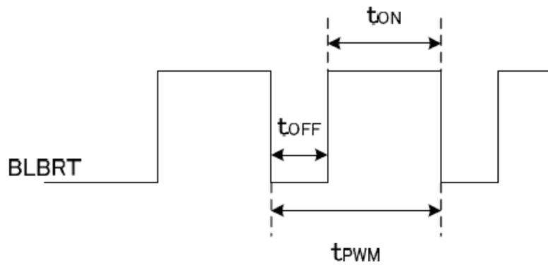
$t_{ON}, t_{OFF} = 50 \mu s$ .
