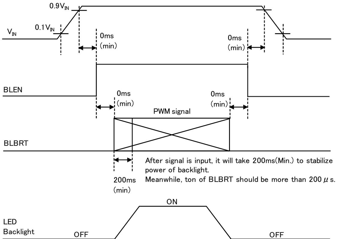
2)  $V_{IN} = 12V$ , Temp. = 25 ,  $D_{PWM} = 100\%$
