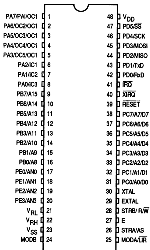
48-Pin DIP Pin Assignments
