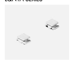
The LQN1A Series is comprised of aircore chip coils having sub-miniature alumina core bobbins. These coils are excellent in high-frequency video and communication applications because of their high Q values at high frequencies and high self-resonant frequencies.
