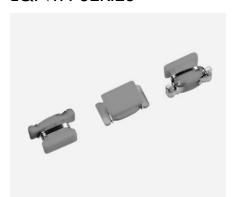
Chip coil LQN1H Series is a wire wound type chip coil using a high frequency ferrite core. Its high Q value at 30MHz ~ 150MHz and low DC resistance are suitable for high frequency resonator circuits use.
