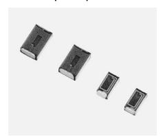
The LQP Series is comprised of chip coils with a tight inductance tolerance, ±2%, achieved in a small chip area. Murata achieves this by forming the coil with precision film technology.
