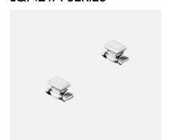
The LQN21A Series consists of air-core chip coils using a subminiature alumina core as a bobbin. The high Q value at high frequencies and high self-resonant frequencies make this coil perfect for use in the high frequency circuits of communications equipment.
