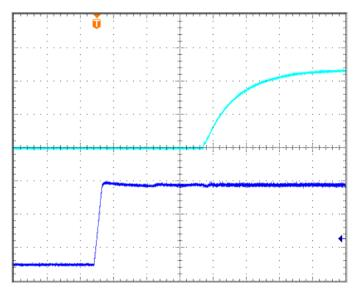
**Figure 7**: Turn-on transient at full rated load current (20 ms/div). Top Trace: Vout; 5V/div; Bottom Trace: input voltage: 20V/div.
