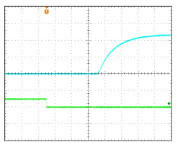
**Figure 5:** Turn-on transient at full rated load current (20 ms/div). Top Trace: Vout: 5V/div; Bottom Trace: ON/OFF input: 5V/div.
