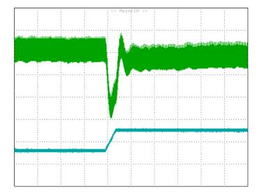
**Figure 8:** Output voltage response to step-change in load current (75%-50% of Io, max; di/dt = 0.1A/µs). Load cap: 100uF Al-Electrolytic capacitor, 10µF tantalum capacitor and 1µF ceramic capacitor. Top Trace: Vout; 100mV/div; Bottom Trace: output current: 10A/div, Time: 200us/div
