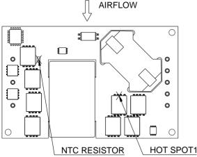
**Figure 21:** \* Hot spot1 and NTC resistor temperature measured point. The allowed maximum hot spot1 temperature is defined at 111  $\mathcal{C}$ .
