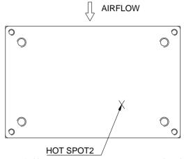
**Figure 23:** \* Hot spot2 temperature measured point. The allowed maximum hot spot2 temperature is defined at 105  $\mathcal{C}$ .
