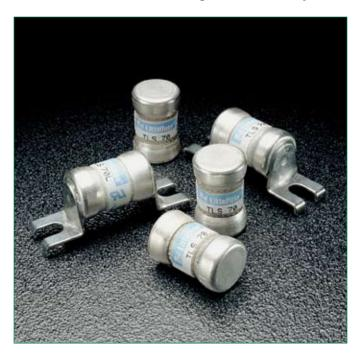
Littelfuse TLS Series fuses are designed specifically for the protection of telecommunications equipment. TLS fuses have been engineered to operate up to 170 VDC to provide current-limiting short-circuit protection for cables and components found in the DC power distribution circuits of telecommunications systems. The compact design and multiple mounting configurations of the TLS series allow it to be used in a variety of applications.
