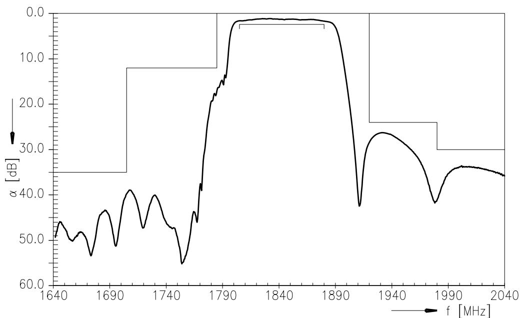
**Transfer function filter 1 (GSM1800) - wideband**
