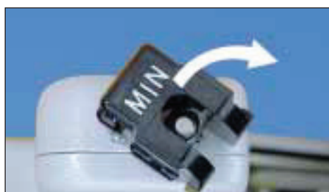
GS2B Tool — Tension Setting Knob
