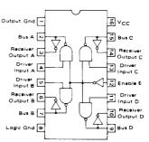
MC3443 0 to 70°C P Suffix - Case 648 Quad Transceivers without termination resistors. Functional equivalent to 75138
