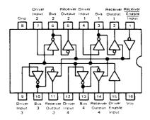
MC8T26/MC6880 0 to +75°C L Suffix — Case 620 P Suffix — Case 648 Quad three-state bus transceiver
