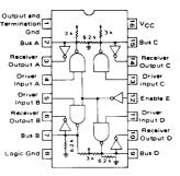
MC3440 0 to 70°C P Suffix — Case 648 Quad Transceivers with 3 Drivers Sharing a Common Enable Input  $R1 = 3.0 \text{ k (to V}_{cc})$  R2 = 6.2 k (to Gnd)
