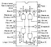
MC3441 0 to 70°C P Suffix —Case 648 Quad Transceivers with all four Common-Enable Input  $R1 = 3.0 \text{ k (to V}_{cc})$  R2 = 6.2 k (to Gnd)
