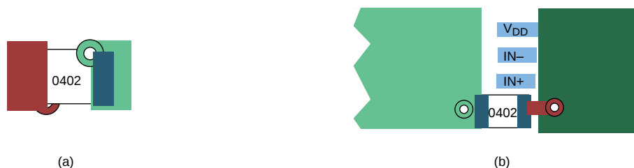
Figure 30. Typical Decoupling Capacitor Layouts
