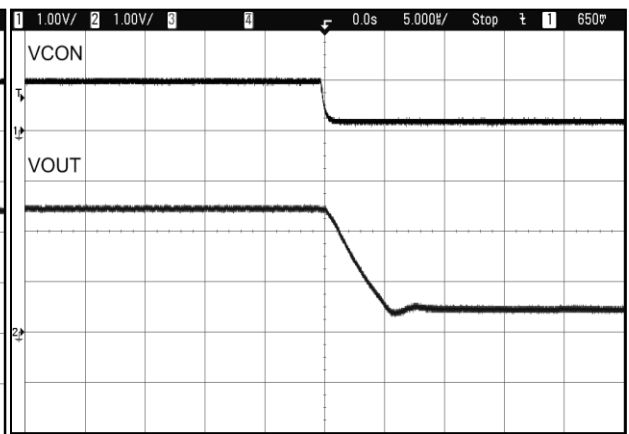
Figure 26. V_{OUT} Falling Transition 2.5 V to 0.5 V, V_{IN} = 3.7\text{ V}
