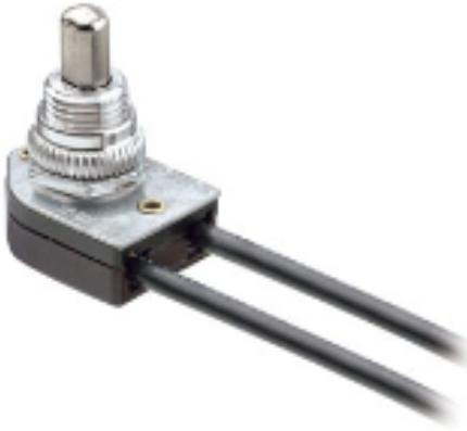
Push button switch, single pole on-off; 1.5A-250VAC, 3A-125V AC-L; male round bushing 3/8-27 by 27/64 inch long thread; two 6 inch black leads 18 AWG AWM TEW 105C 600V, free ends stripped 3/4 inch.
