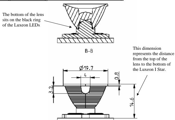
Dimensions tolerance is +/-0.2mm
