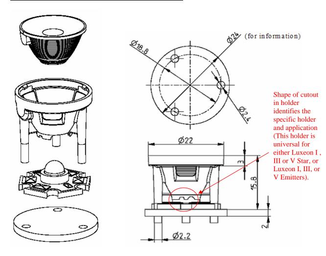
Dimensions tolerance is +/-0.2mm
