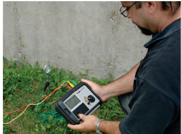
Model DET3TD shown performing the classic fall-of-potential test method.
