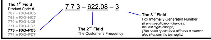
This example, FXO-PC536R-622.08 = LVPECL Output, Ceramic, 5 x 3.2mm Package, 3.3V, ±25 PPM Stability, -40 to +85°C Temperature Range, at 622.08 MHz
