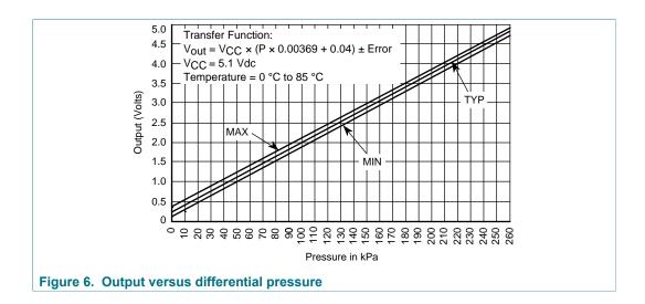
$V_{OUT} = V_{CC} \times (P \times 0.00369 + 0.04) \pm (Pressure Error \times Temp. Factor \times 0.00369 \times V_{CC})$ Nominal transfer value:
