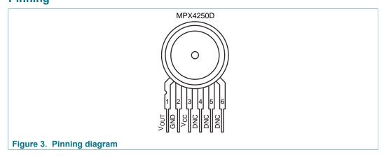
0 to 250 kPa, Differential, gauge pressure sensor, on-chip signal conditioned, temperature compensated and calibrated
