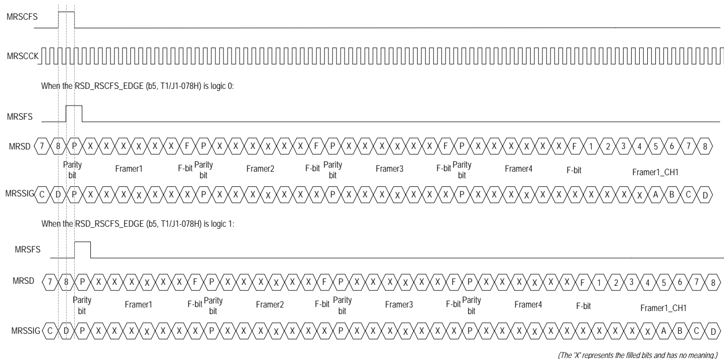
Figure 34. T1/J1 Receive Multiplexed Mode - Functional Timing Example 2
