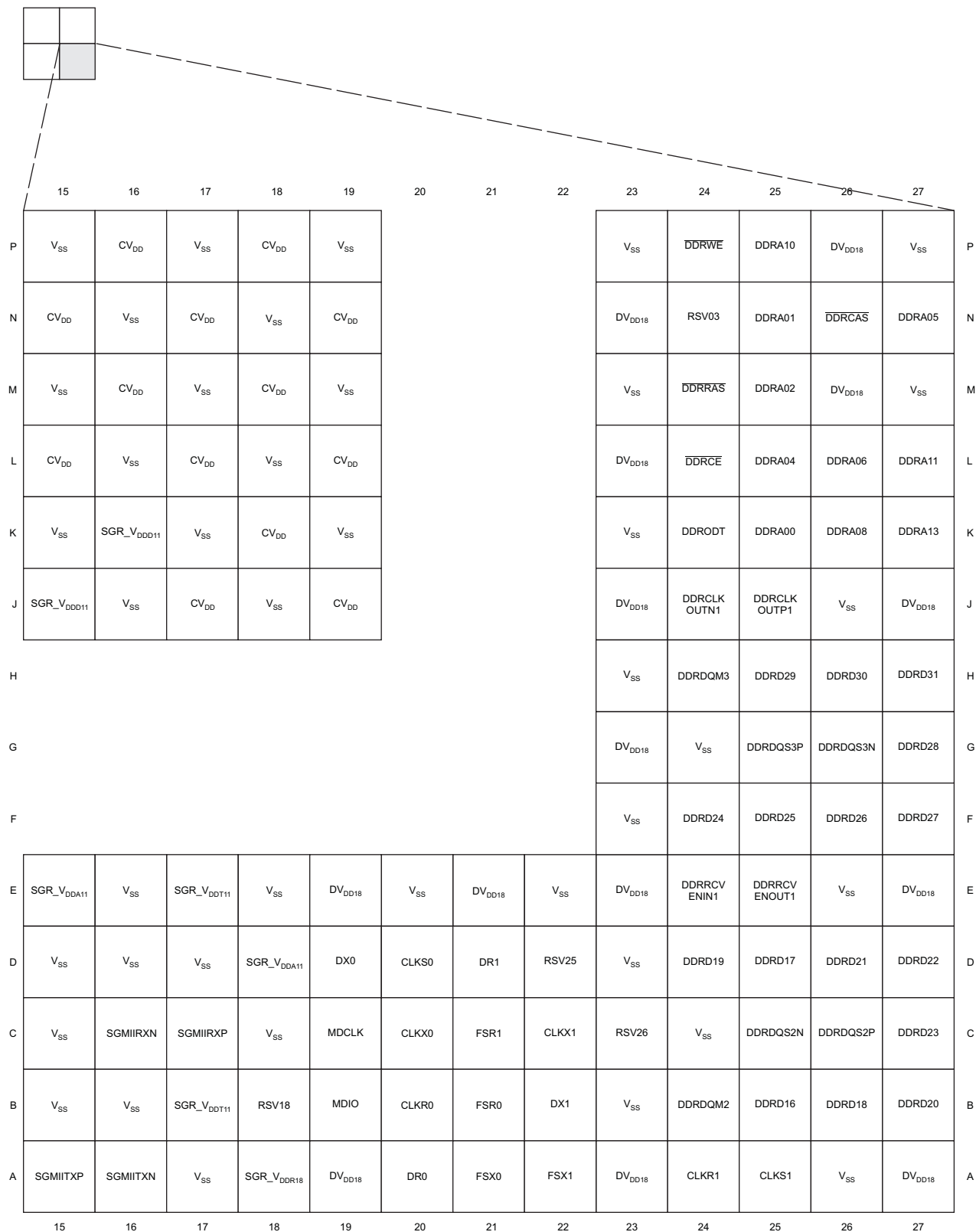
Figure 2-4. C6474 Pin Map (Bottom View) [Quadrant C]
