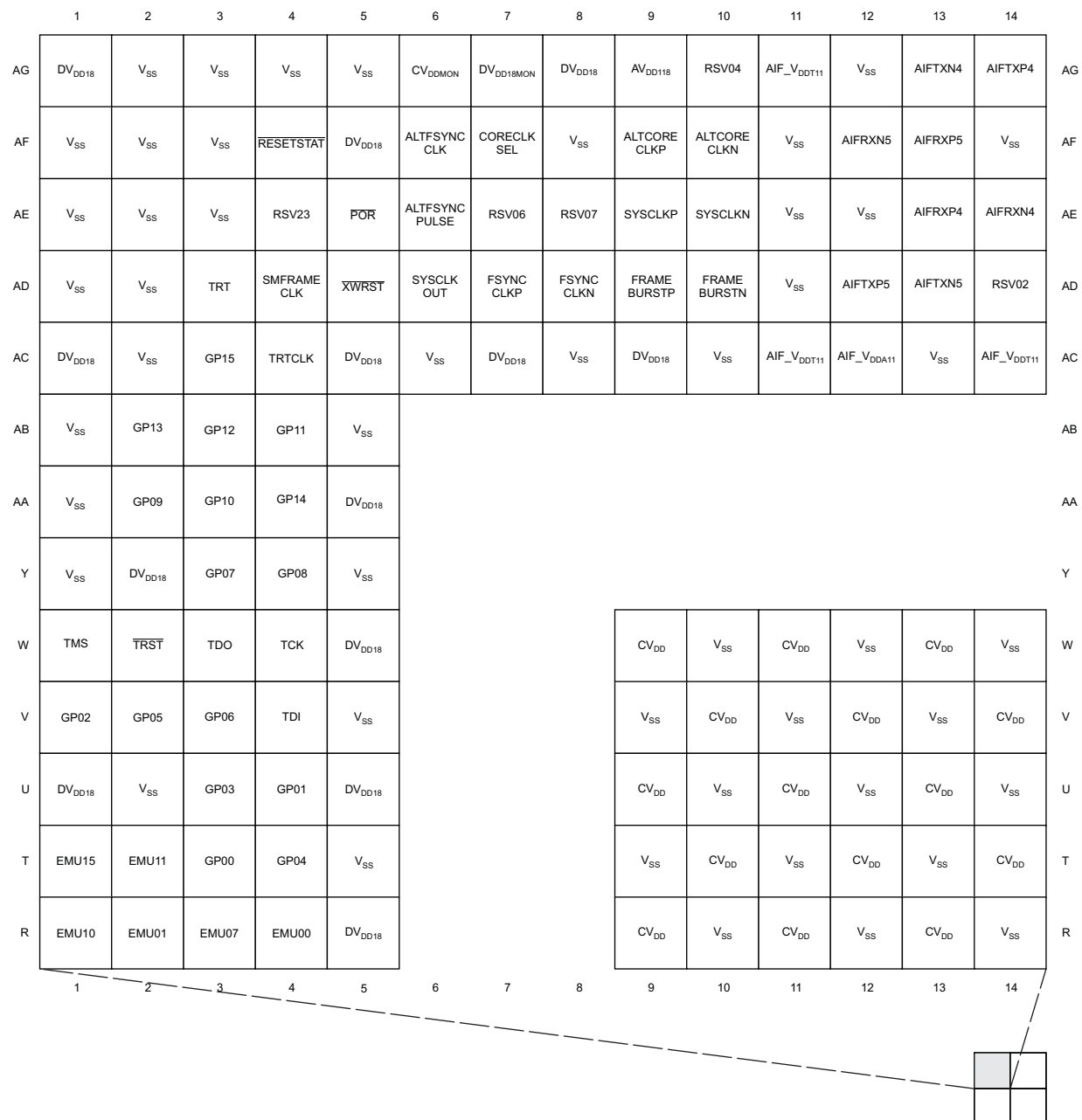
Figure 2-2. C6474 Pin Map (Bottom View) [Quadrant A]
