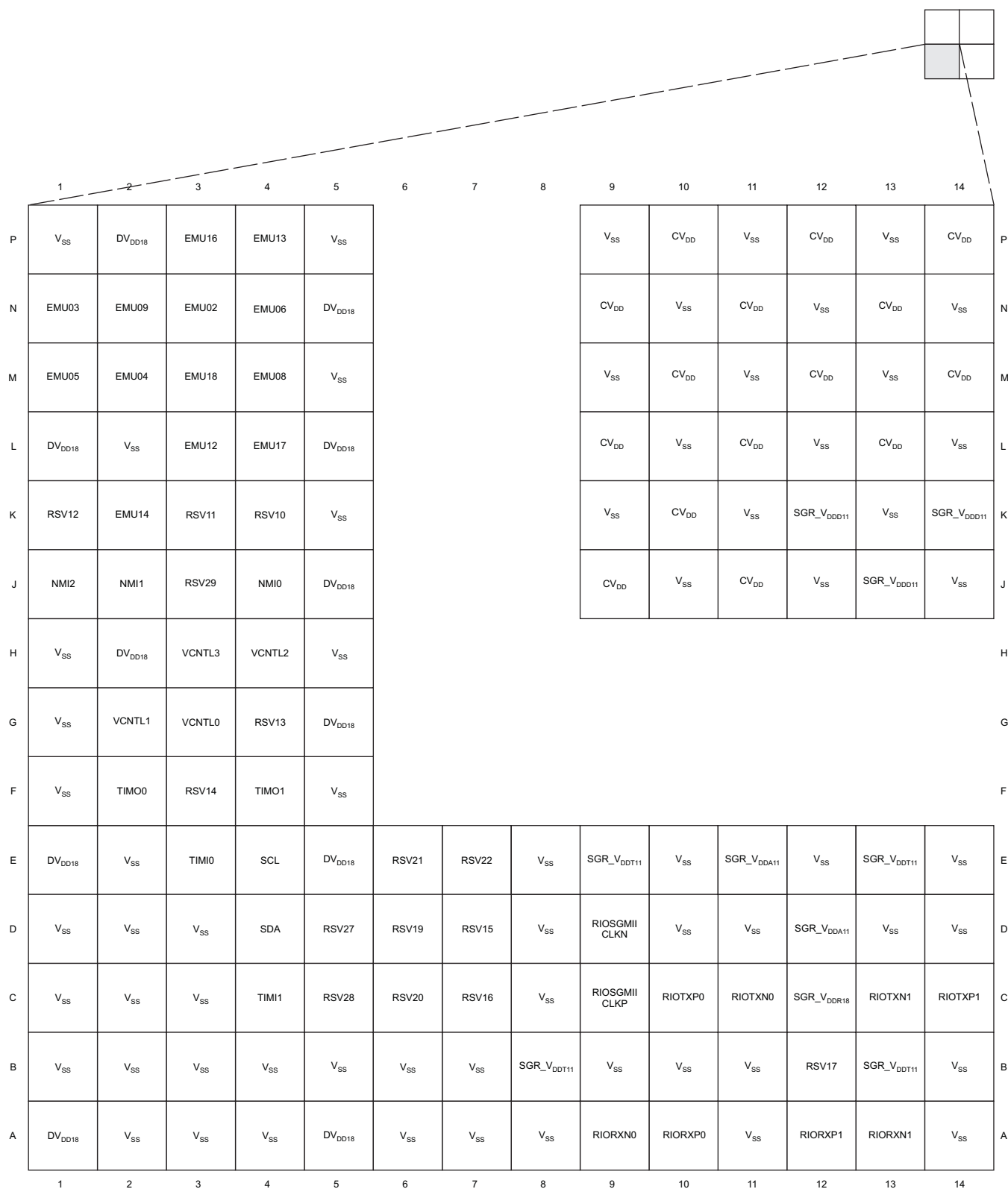
Figure 2-5. C6474 Pin Map (Bottom View) [Quadrant D]
