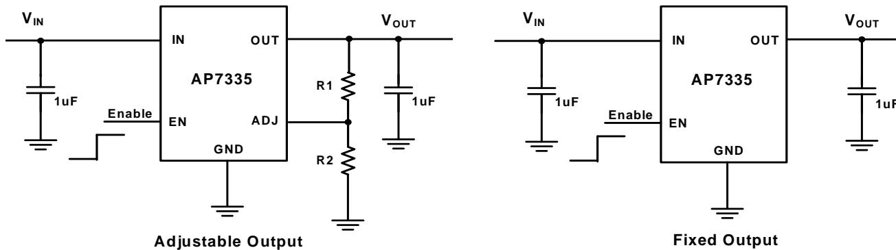
$$V_{OUT} = V_{REF} \left( 1 + \frac{R_1}{R_2} \right) \text{ where } R_2 \leq 80\text{K}\Omega$$
