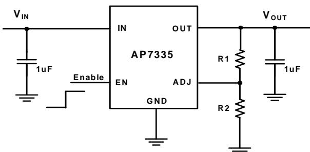
The output voltage is calculated by:
