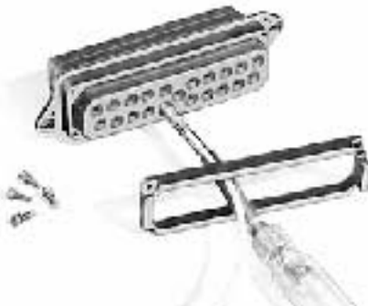
Inserting Coaxial & #12 Contacts
