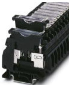
Fuse modular terminal block, without fuse plug, Connection method: Screw connection, Cross section: 0.5 mm<sup>2</sup>- 16 mm<sup>2</sup>, AWG: 20 - 6, Nominal current: 10 A, Nominal voltage: 500 V, Width: 10.2 mm, Fuse type: G / 5 x 20 / 5 x 25 / 5 x 30 / 6.3 x 32, Fuse type: Glass, Mounting type: NS 35/7,5, NS 35/15, NS 32, Color: black
