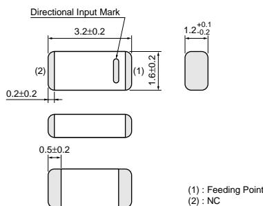
Terminal of "NC" should be connected to the floating land.
