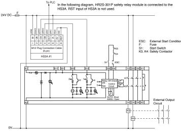
For details of HR2S-301P safety relay module, see the instruction sheet.
