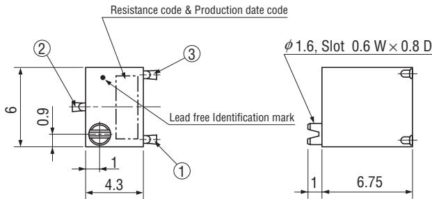
Unless otherwise specified, tolerance :  $\pm 0.3$  (Unit: mm)
