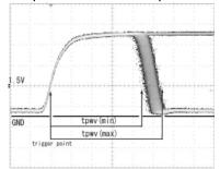
Vertical axis: 1 V/div., Horizontal axis: 5 ns/div. (Ta=25 °C, Vcc=5.25 V, Pi= -26 dBm, RL=50 k $\Omega$ , CL=15 pF, 45.2 Mbps)
