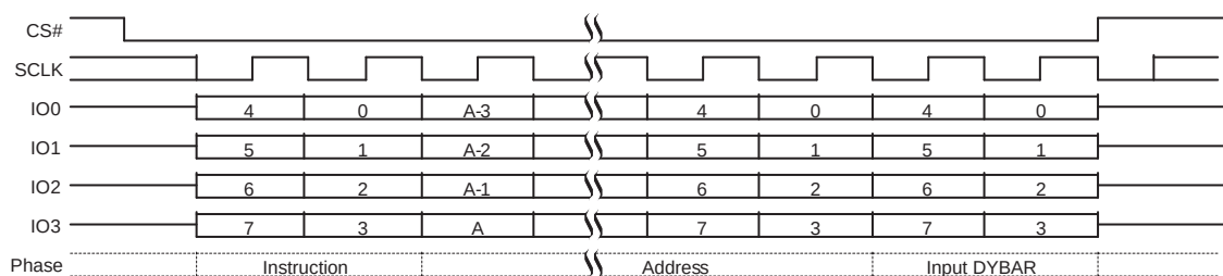
Figure 10.63 DYBWR QPI Mode Command Sequence
