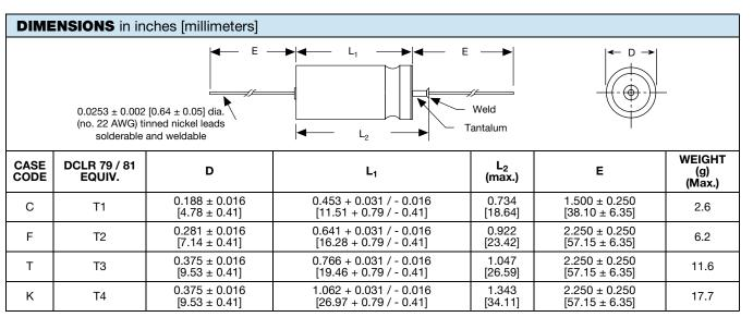
• For insulated parts, add 0.015" [0.38] to the diameter. The insulation shall lap over the ends of the capacitor body.
