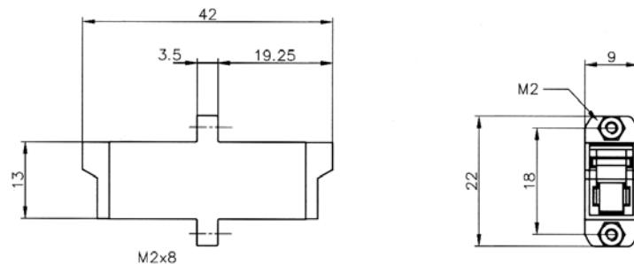
The E2000 connector and adapter have set the standard for optical fibre interconnect. With a shutter on both the connector and adapter to prevent laser eye damage the E2000 offers features no other connector can match. The E2000 also has a latched lever mechanism to prevent accidental disconnection.
