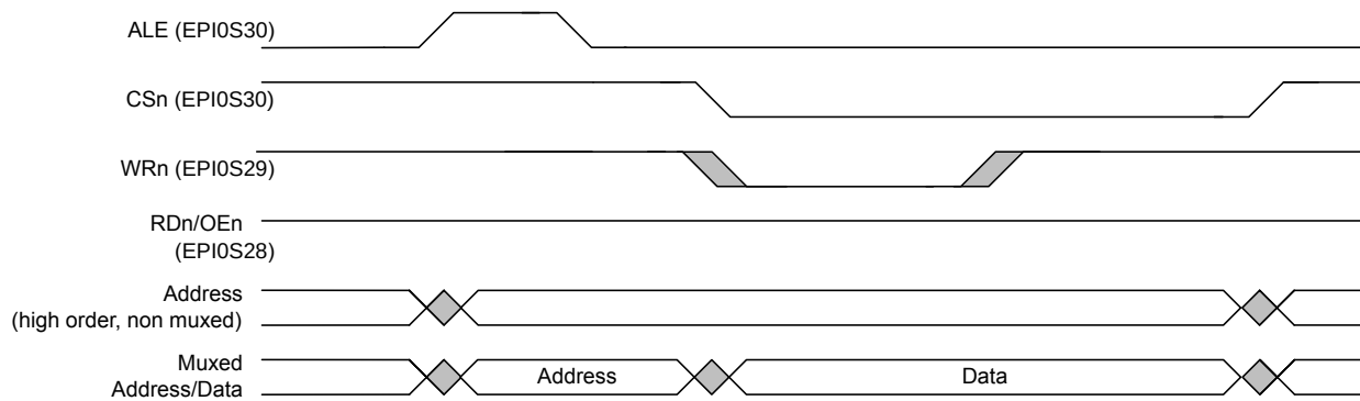
Figure 10-7. Host-Bus Write Cycle with Multiplexed Address and Data, MODE = 0x0, WRHIGH = 1, RDHIGH = 1
