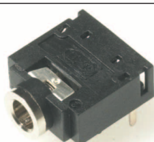
JYO-39-3P stereo unswitched 3.5mm Jack Socket. JYO-39-5P stereo switched version. Right angle PCB mounting.
