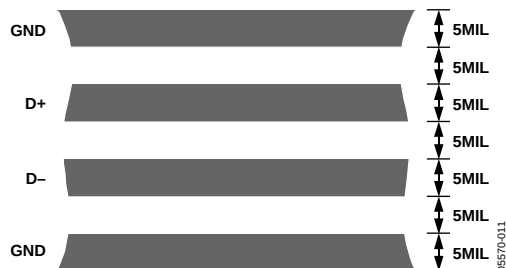
Figure 22. Typical Arrangement of Signal Tracks
