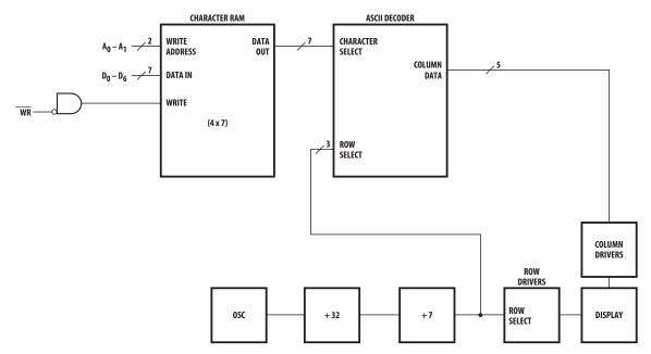
Figure 2. Display internal block diagram.
