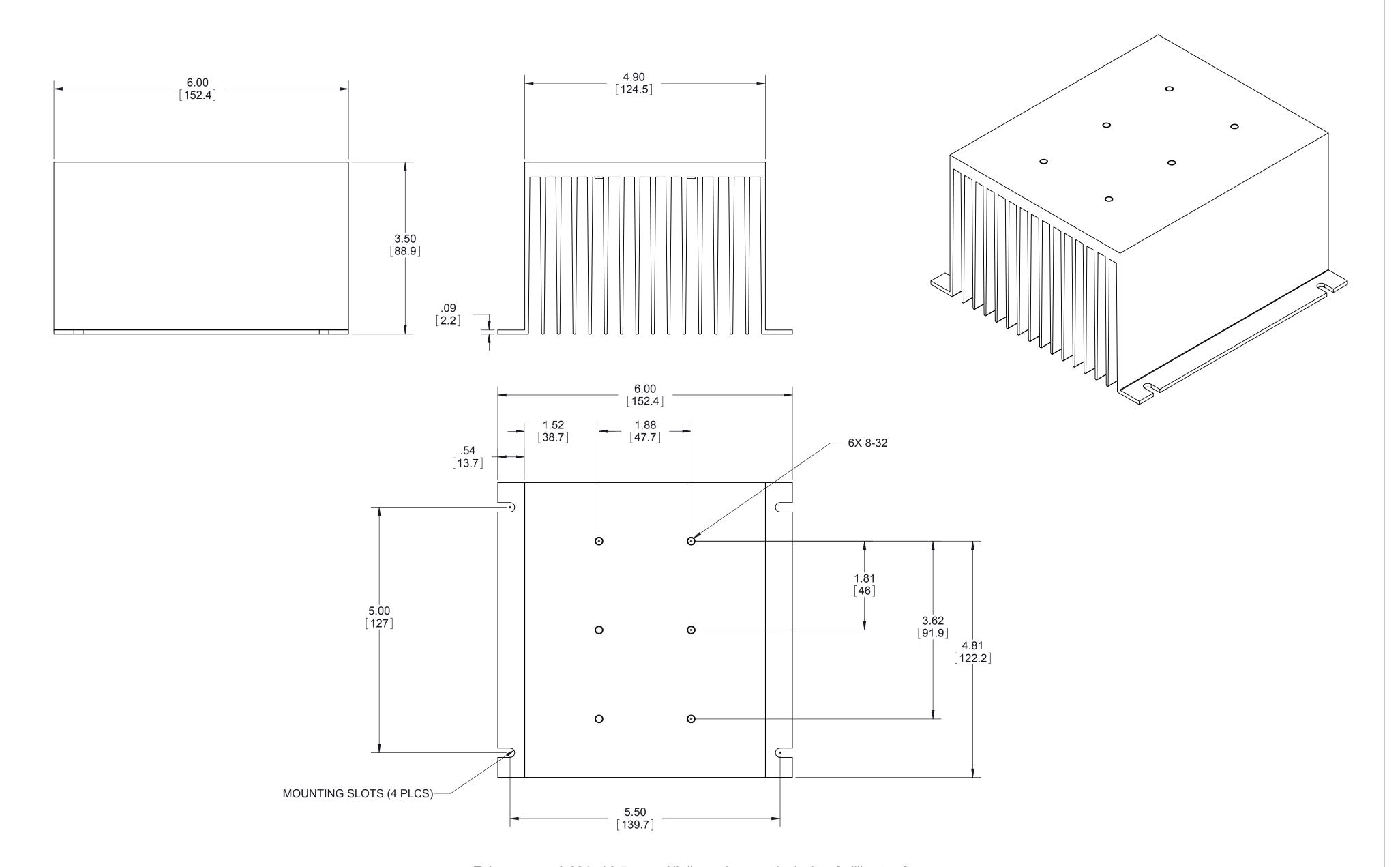
Tolerances: ± 0.02 in / 0.5 mm. All dimensions are in: inches [millimeters]
