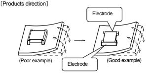
Products shall be located in the sideways direction to the mechanical stress.
