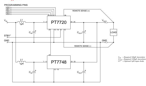
Output Capacitors: The PT7720 series requires a minimum output capacitance of 1200µF for proper operation. Do not use Oscon type capacitors. The maximum allowable output capacitance Is (57,000 ÷ Vout)µF, or 15,000µF, whichever is less.
