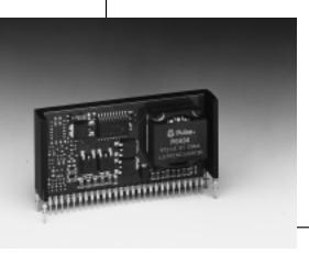
The PT7748 is a new high-performance 17 Amp "Current Booster" for the PT7720 Series housed in a 27-pin SIP package. Multiple PT7748 boosters will operate in parallel with the PT7720 Series boosting output current in increments of 17A. Combinations of PT7720 and PT7748 current boosters can easily supply enough power for virtually any multiple megaprocessor application.
