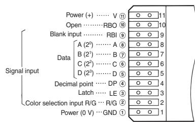
**Note:** 1. The latch terminal on ±1. Display Units is provided only on Dynamic Output Models.
