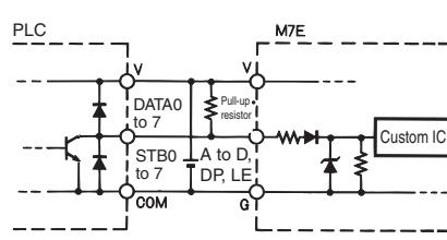
Note: 1. Supply 24 VDC only. The PLC does not operate with the M7E Negative Logic Model.
