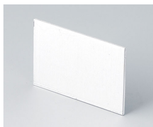
B6112112 Rear panel Aluminum matt anodized 1.66"x1.17"x0.04"
