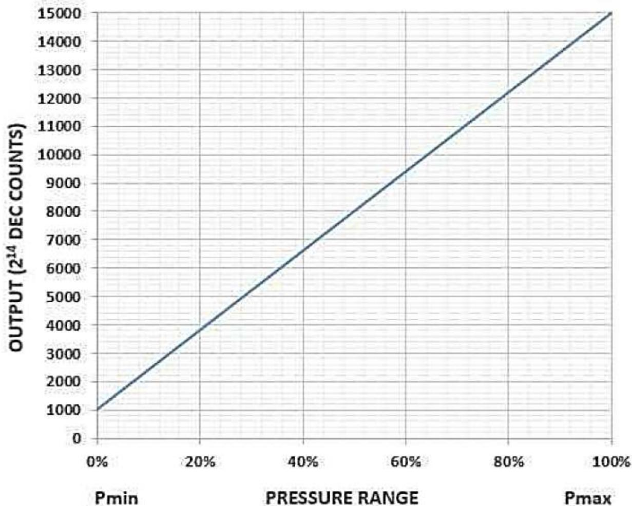
$$\text{OUTPUT (DECIMAL COUNTS)} = \frac{15000 - 1000}{P_{\max} - P_{\min}} \times (P_{\text{applied}} - P_{\min}) + 1000$$
