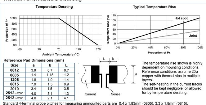
0.4 x 2.8mm (1206), 1.2 x 4.5mm (2010) and 1.5 x 5.8mm (2512). All probe location tolerances ±0.02mm.
