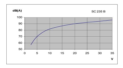
All measurements are made at 1 meter in free air at 21°C.
