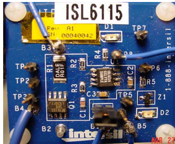
FIGURE 18. ISL6115 EVAL BOARD PICTURE
