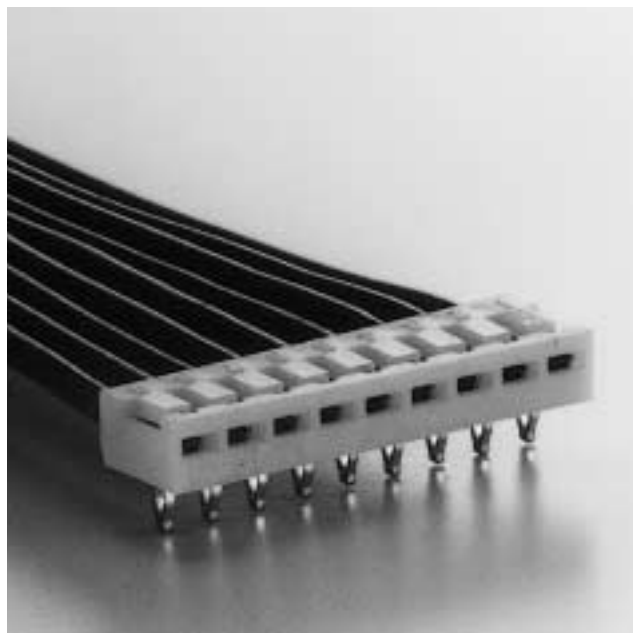
Side entry type board-in connector, with a mounting height of only 2.8mm (.110") and a thickness of 4.9mm (.193").
