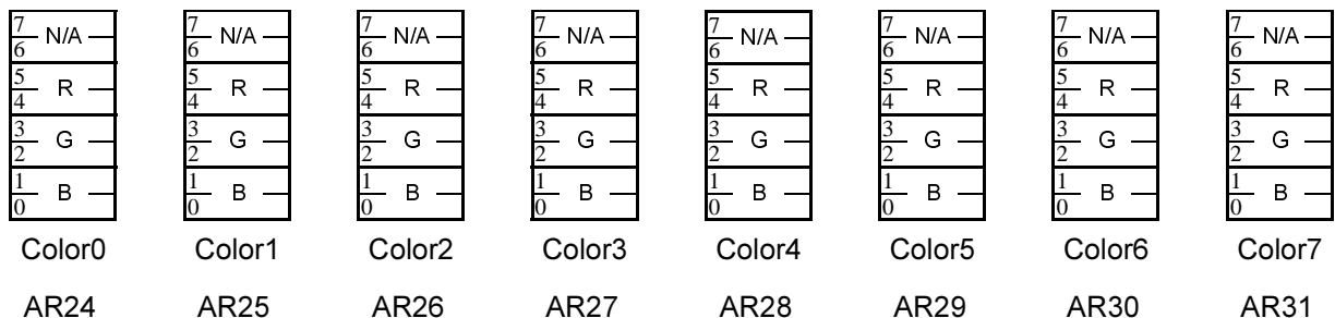
Figure 24 Programmable Palette Control at AR Register
