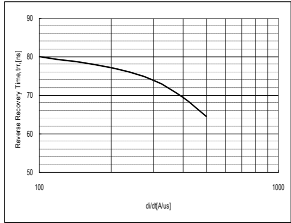
Fig. 2 : Typical Reverse Recovery Time vs. -di/dt
