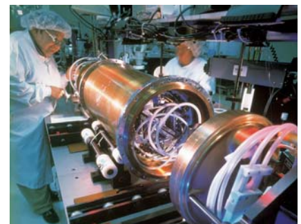
Telecommunications Undersea Cable Repeater
