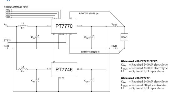
Output Capacitors: When used with a PT7771 or PT7772, the PT7746 requires a minimum ouput capacitance of 2400µF. When used with a PT7777, the PT7746 requires a minimum ouput capacitance of 680µF for proper operation. Do not use Oscon type capacitors. The maximum allowable output capacitance is 30,000µF.
